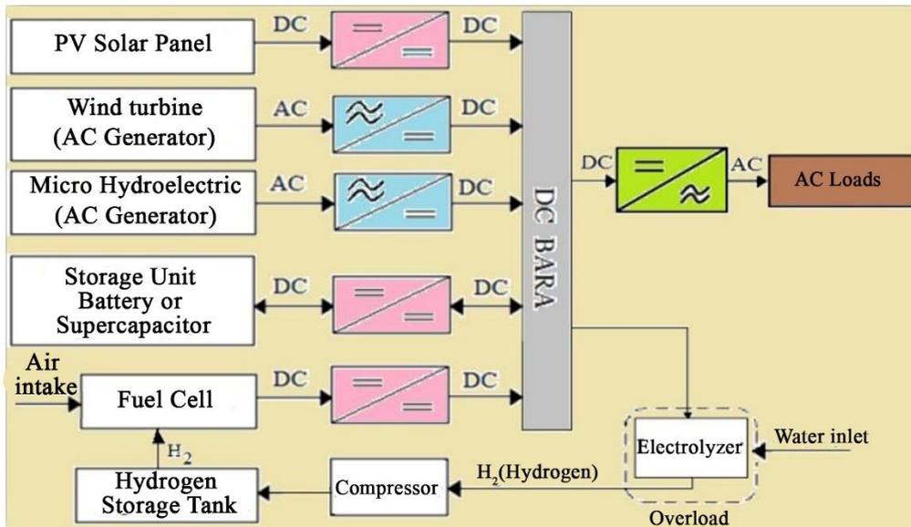
Figure 78. Components of microgrids
