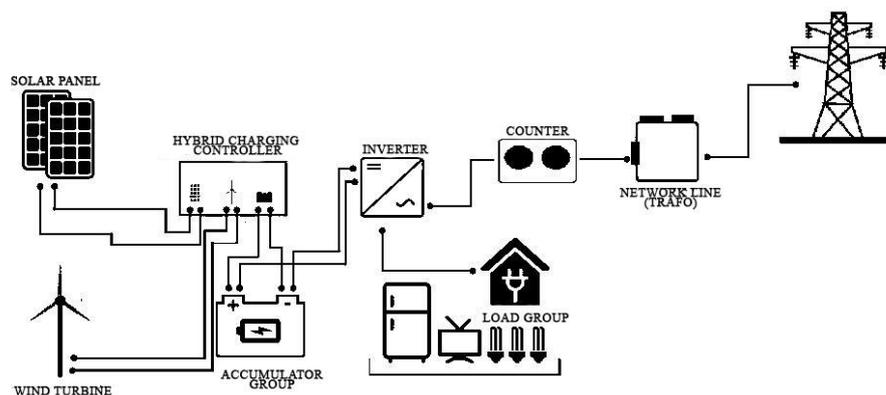
Figure 28. Hybrid PV system [30]
