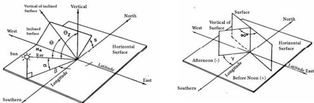
Figure 16. Angles formed by solar radiation on the Earth's surface.
