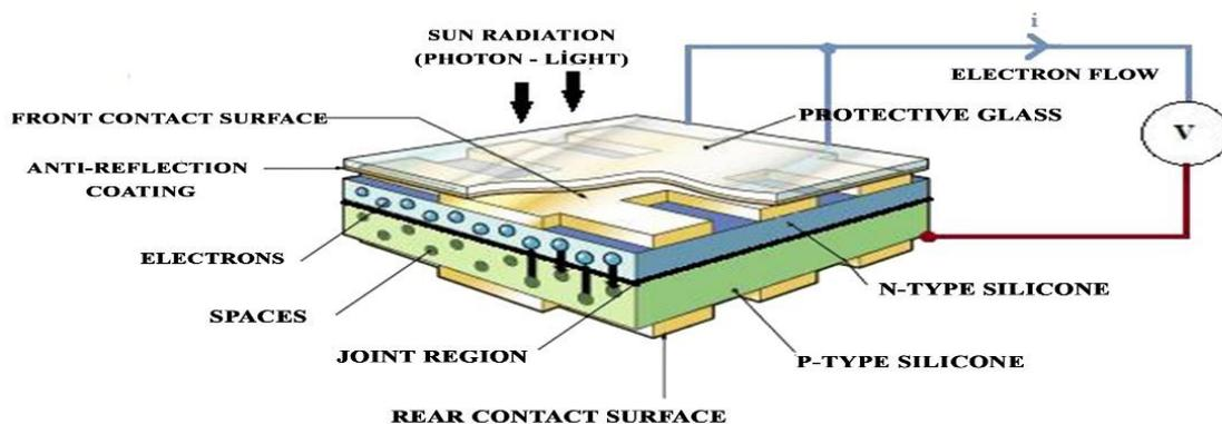
Figure 29. Photovoltaic cell structure and working mechanism [30]
