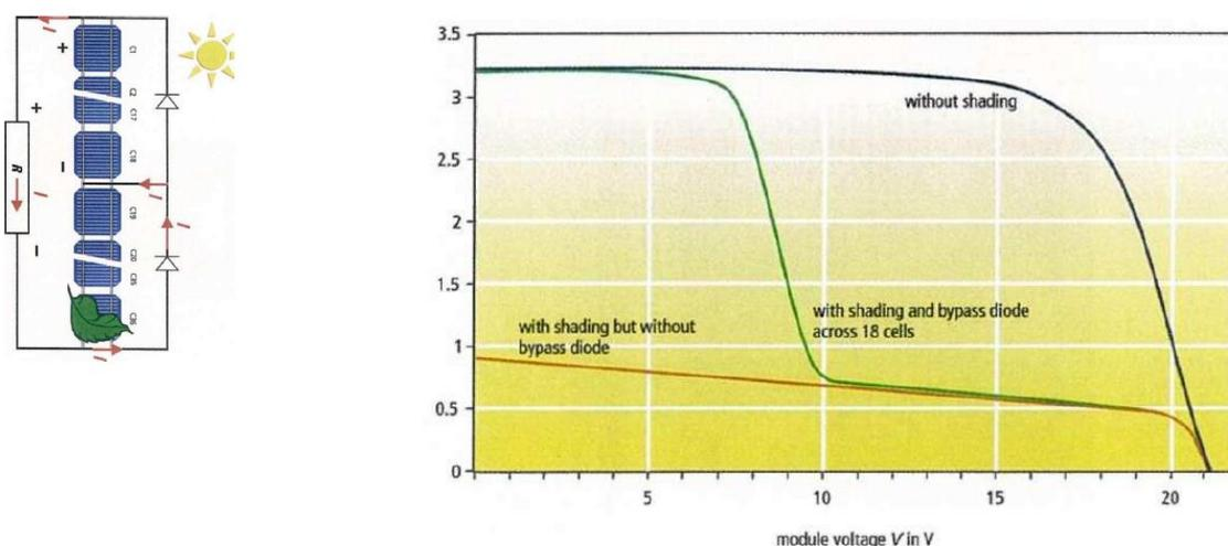
Figure 67. Module I / V Graph Change with and without Bypass Diode When Shadow Falls on the Module
