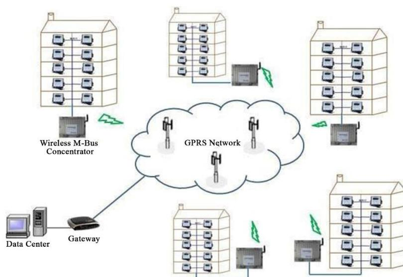
Figure 80. MBUS Meter Reading System
