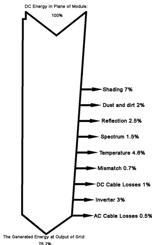
Figure 39. Percentages of Module Energy Losses
