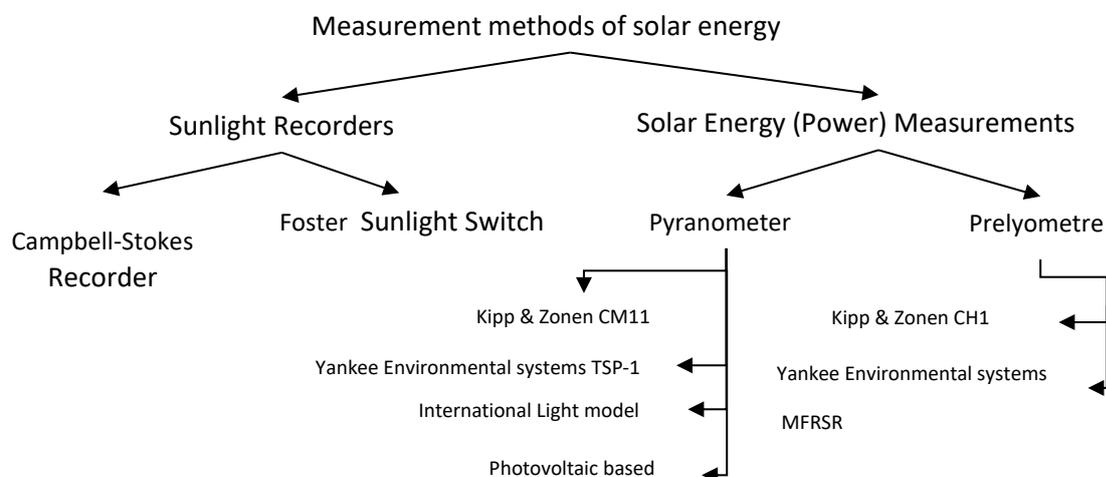
Figure 7. Classification of solar energy measurement methods
