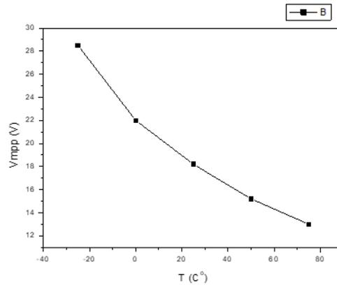
Figure 68. Variation of V<sub>mpp</sub> Value with Temperature Under Constant Light Intensity
