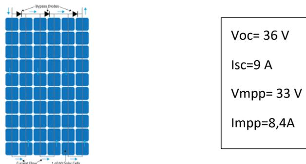
Figure 69. A Panel Composed of 60 Cells
