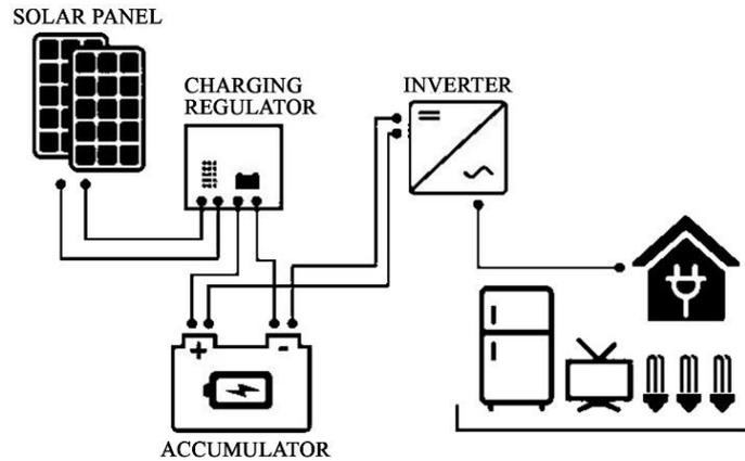
Figure 27. Off-grid PV system [30]
