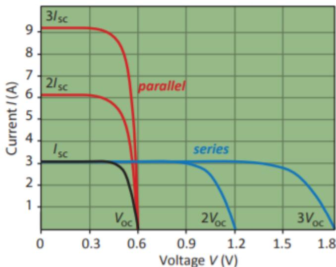
Figure 35. I-V curves of solar cells connected in series and parallel [37]
