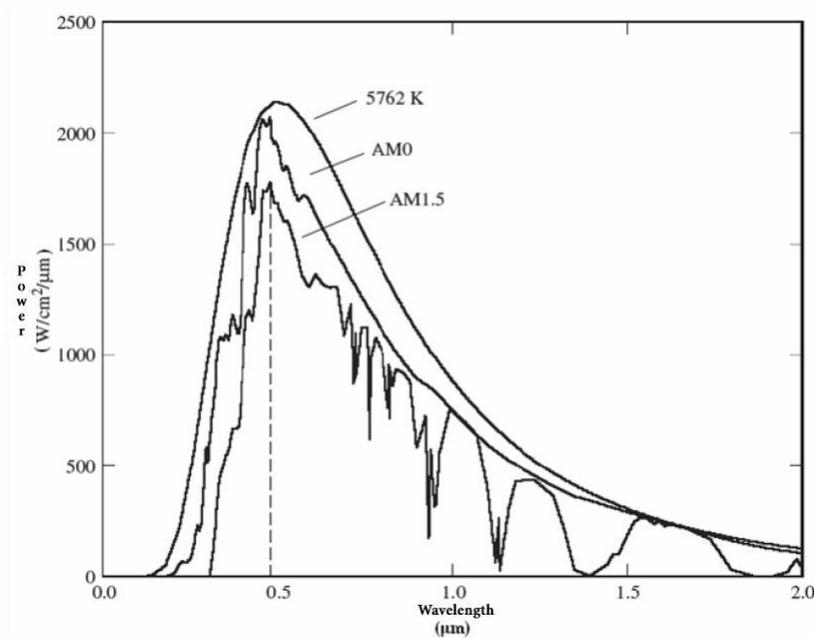
Figure 6. Comparison of the solar surface irradiance spectrum with AM0 and AM1.5 spectra
