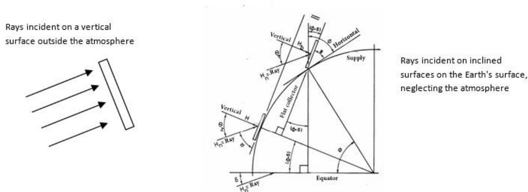
Figure 17. Calculation of total rays incident on inclined surfaces on the Earth's surface.
