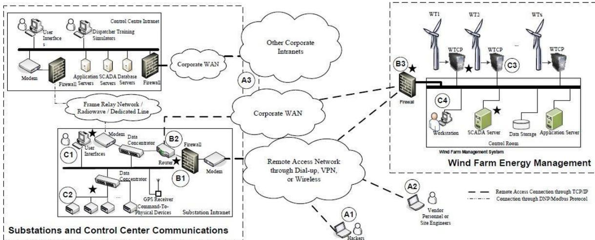
Figure 77. SCADA Infrastructure and Network Connectivity Between Substation-Level Network, Control Centers, and a Wind Farm Management System
