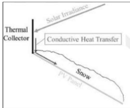
Figure 57. Thermal Collector
