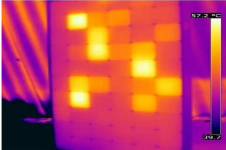
Figure 52. Thermal Camera Imaging of a Solar Panel and its Temperature Value
