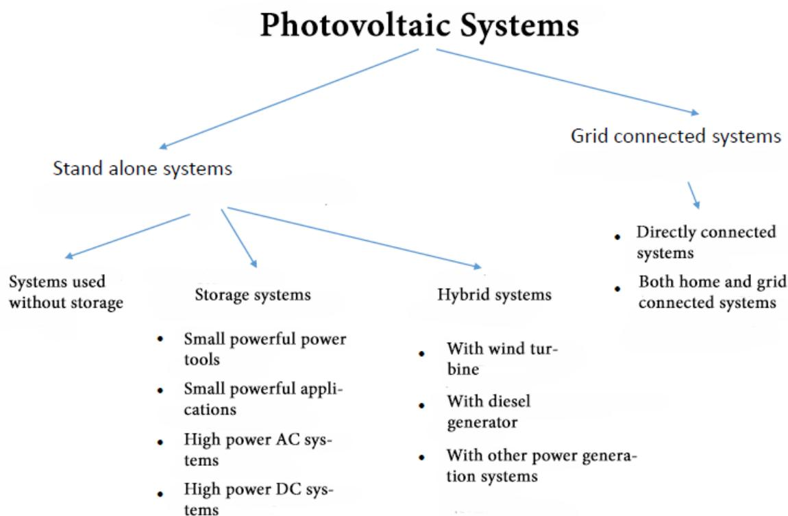
Figure 18. Areas of use of photovoltaic systems
