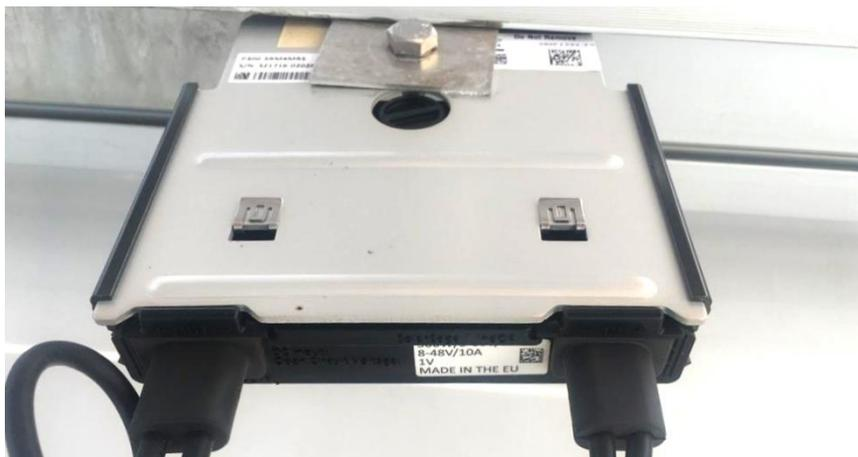
Figure 33. Charge Control Unit
