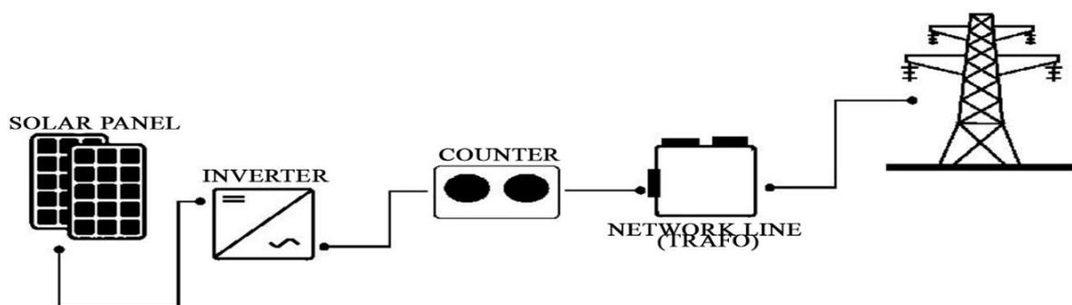
Figure 26. Grid-connected PV systems [30]
