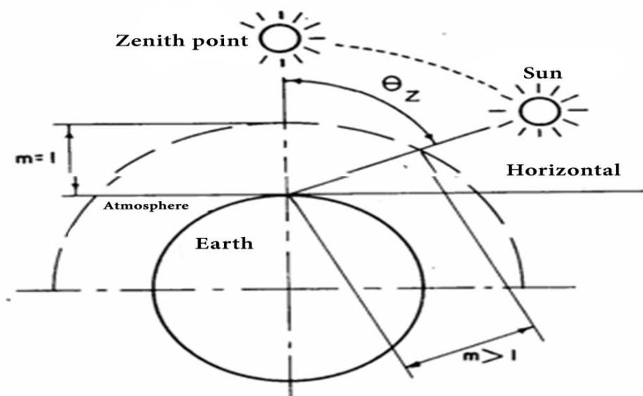
Figure 5. Change in Air Mass as the Sun's rays come to the Earth's surface at different angles
