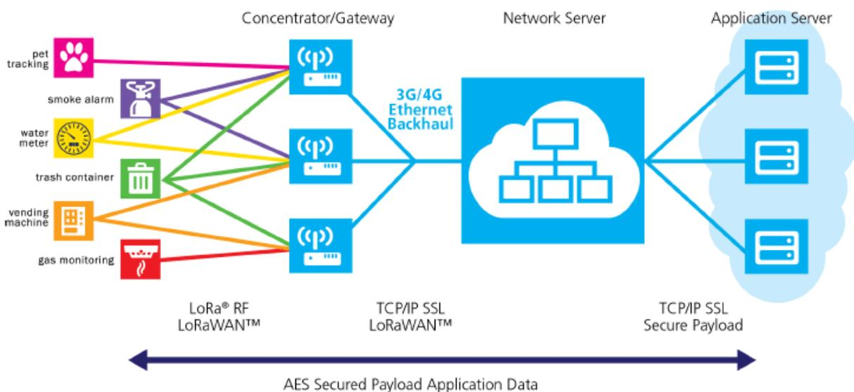
Figure 81. Wireless LoRa Network Management System
