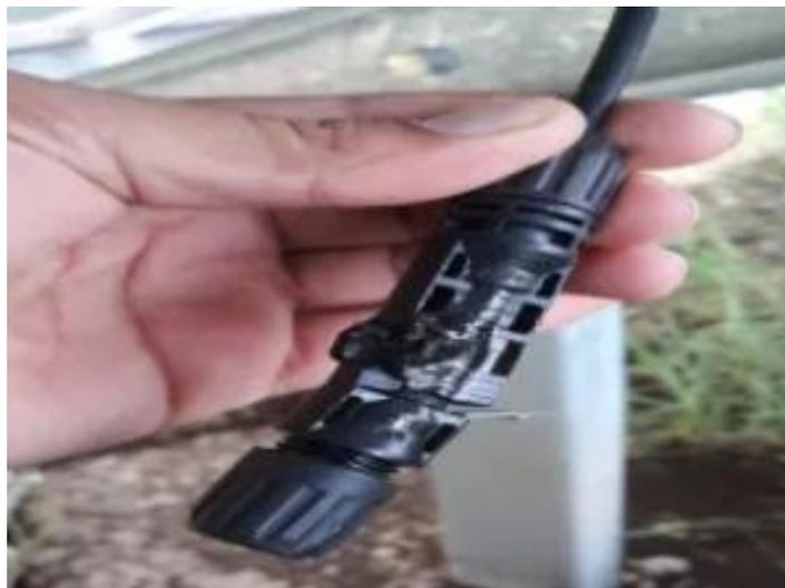
Figure 53. Connector That Burnt Out Due to Incompatibility
