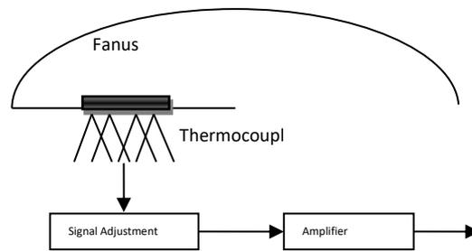
Figure 8. Schematic representation of a pyranometer
