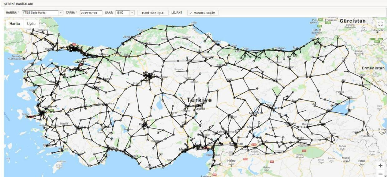
Figure 74. 154KV transmission line network
