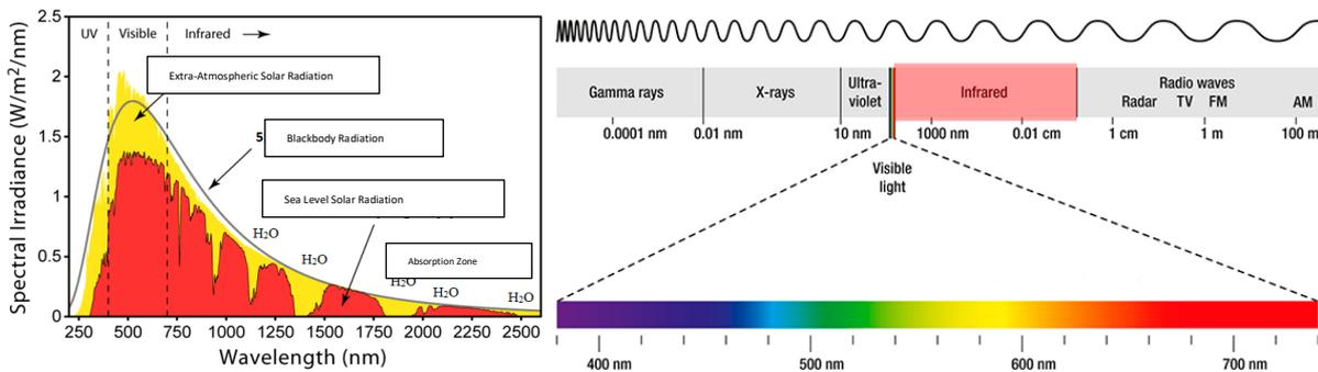
Figure 1. a) Intensity distribution of the rays emitted from the Sun according to wavelength, b) Naming the rays coming to the earth's surface according to the wavelength
