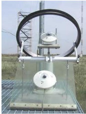
Figure 11. Measuring Reflection Diffuse and Direct Solar Radiation.
